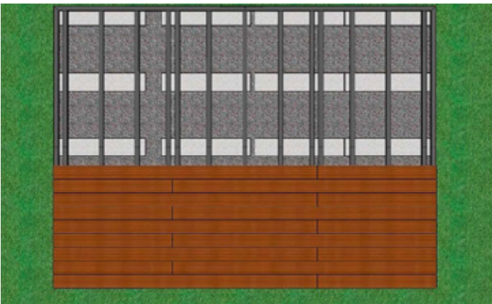
Substructure, substructure and deck with offset joints. Centre-to-centre dimensions: 100-400-400...400-100-400...400-400-100 mm
